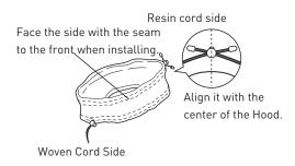
2. Attaching the Face Guard to the inside frame of the Hood.
