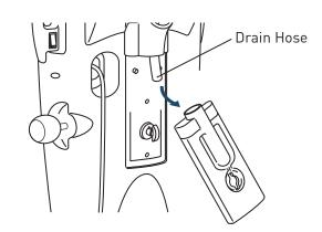
9 Empty the water in the internal section after operations are completed.
