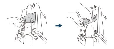
12 Drain the water tank after use.
