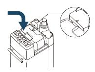
1 Insert the flexible hose into the exhaust nozzle.
